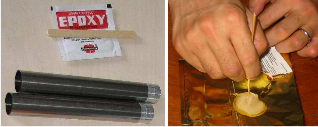
Figure 10: Glue, Mixing Tubes and Inlet Spatula
