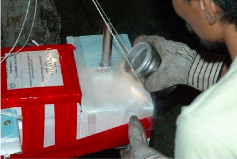
Figure 14: Filling the CFH Cryogen Compartment with Cryogen
