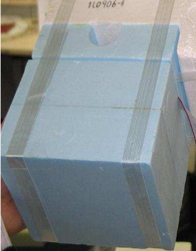
Figure 9: CFH Battery Pack in Final Assembly
