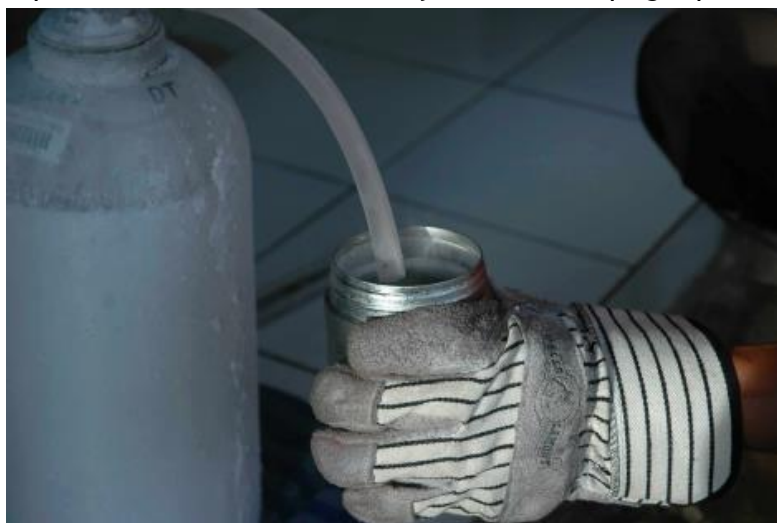
Figure 13: Filling the Cryogen Transfer Cup from a Cryogen Cylinder Equipped with a Dip Tube
