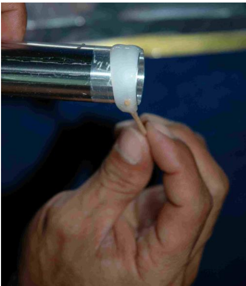
Figure 11: Applying Glue to the Inlet Tube Ring
