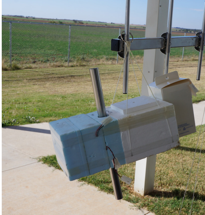
Figure 7. CFH package combined with IMet radiosonde.
