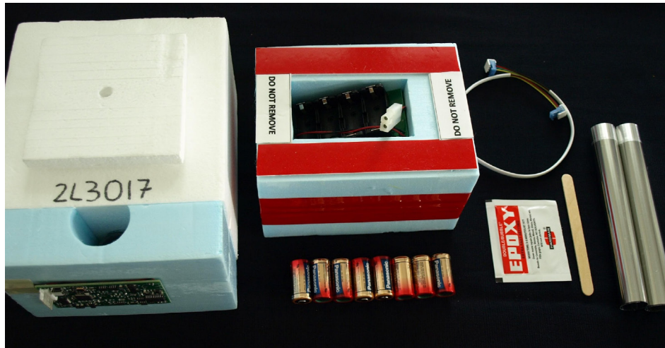
Figure 6. CFH components including battery compartment and air-inlet tubes.
