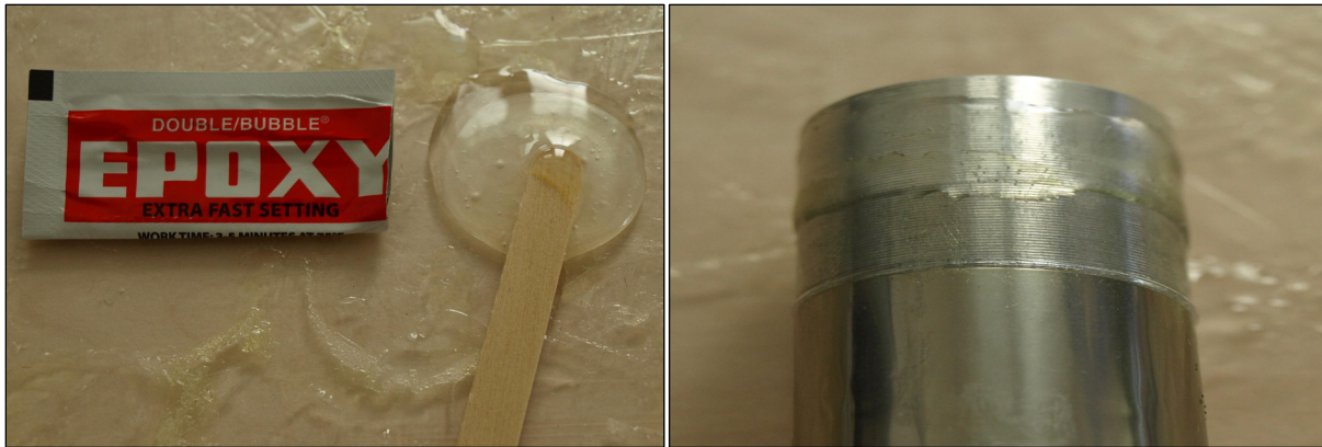
Figure 9. Attaching the air-inlet tubes with epoxy glue.
