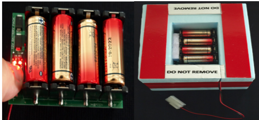
Figure 8. The battery compartment for the CFH, with the battery state lights on the left. Right: The battery compartment placed inside the foam box.
