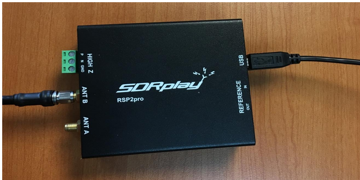
Figure 3. Connections to the SDRplay radio. The cable from the preamp must go to the ANT D connector on the radio.
